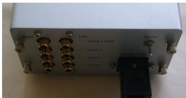
line input/output from RCA pin jacks
